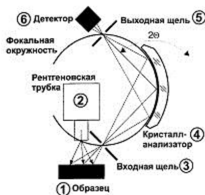
Fig. 2. X-ray fluorescence spectrometer, a scanning scheme
