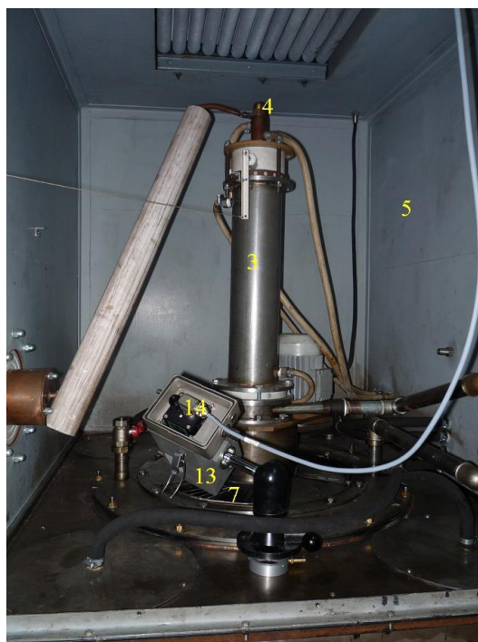
Fig.2 The photo of a laboratory plasma stand "Plasma module based on high-frequency generator VCHG8-60/13-01" with installed gas analyzer «Quintox» KM9106
