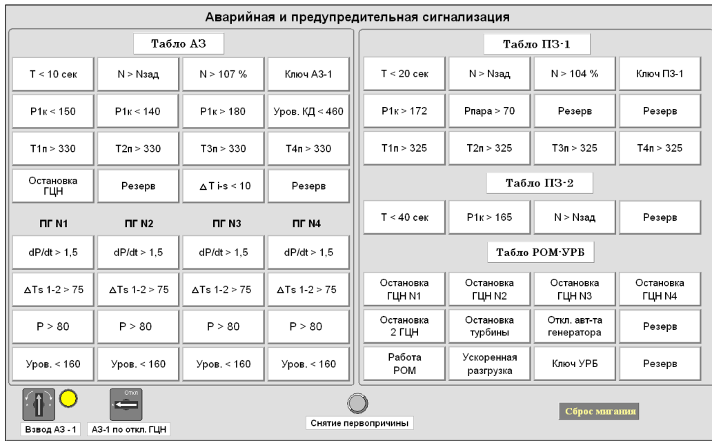
Fig. 2. Display «Emergency and warning system» of WWER-1000.
