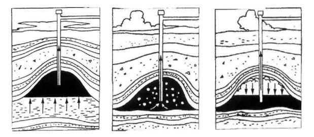
*Fig.6. Drive Mechanisms:* 1. water drive 2. dissolved-gas drive 3. gas-cap drive
