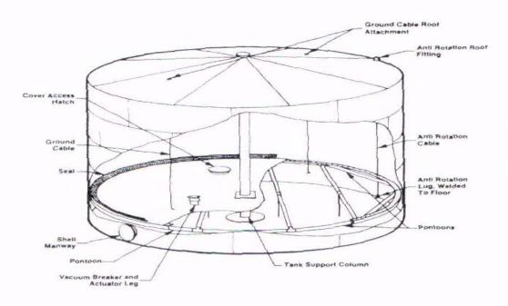
Fig. 2. Typical arrangement of internal floating roof
