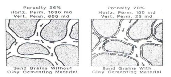
Fig. 4. Effects of clay cementing material on porosity and permeability
