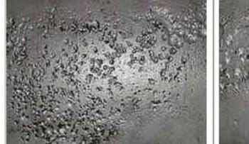
Fig 1: An example of general deep pitting corrosion with some pits joining to form larger pits and interconnected pitting.
