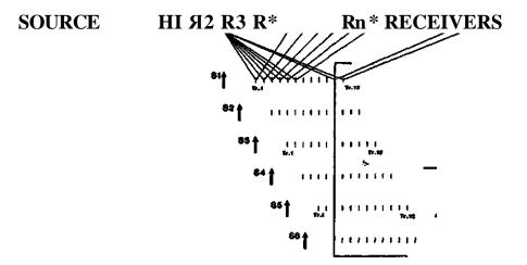
12 End-on pattern channels used for simplicity Fig. 2. Common depth point field geometry
