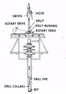
Fig. 7. Schematic of rotary system
