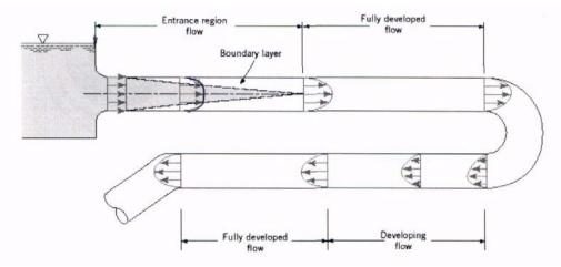
*Fig. 4. Entrance region, developing flow, and fully developed flow in a pipe system*
