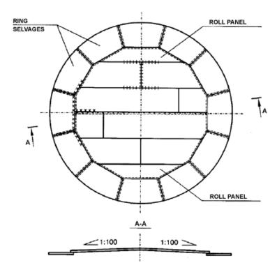
Fig. 5. Conical selvaged bottom
