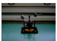
Contrarily to the beam in an ordinary balance, the **beam** in a torsion balance **resolves** in a horizontal plane and is reflected from a position corresponding to the torsionless condition of the **suspension wire** by the unbalance of horizontal forces acting on it.
