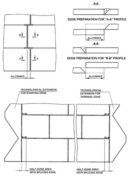
Fig. 3. Wall panels (reservoirs volume over 5000 cub. cm.)
