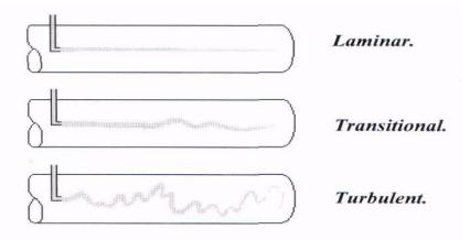
Fig. 3. Fluid Flow in a Pipe
