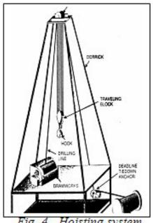
Fig. 4. Hoisting system
