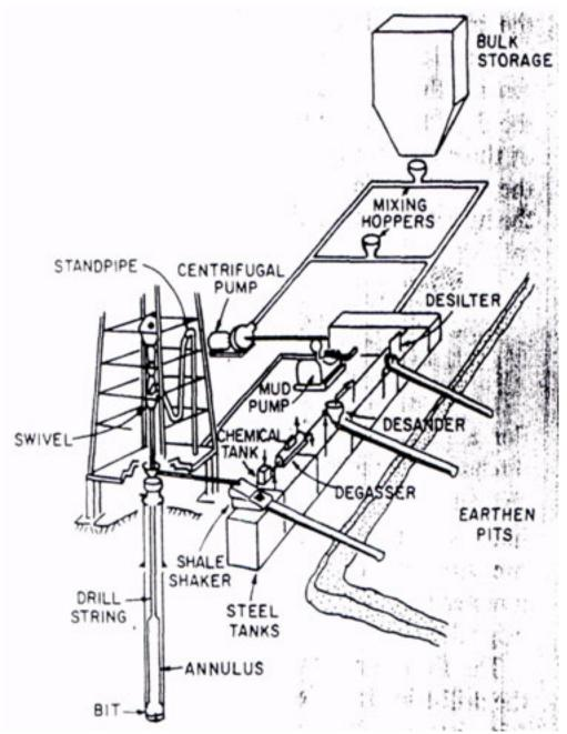
Fig. 8. Schematic of example rig circulating system
