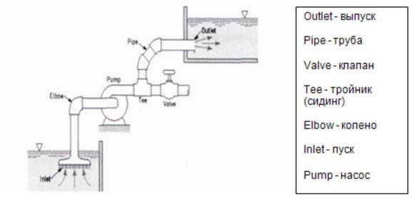
Fig. 1. Typical pipe system components
