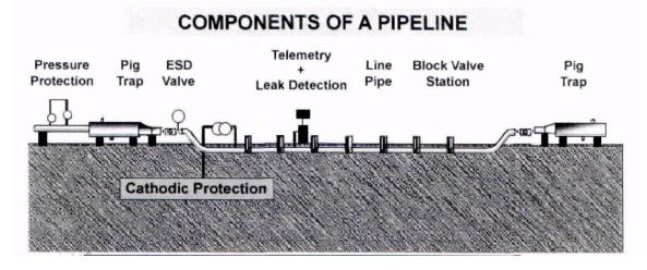
Fig. 3. Components of a pipeline
