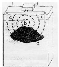
Electrical survey An ore deposit (a) affects natural ground currents. (b)flowing between buried electrodes. (c)millivoltmeter. (d)registers voltages at the electrodes
