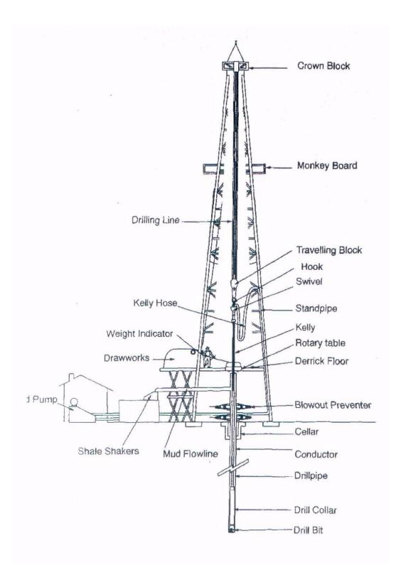
Fig. 2. Drilling rig components
