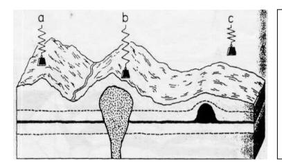
**a.** Normal gravimetric reading.
