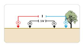
In resistivity procedures not only the potential difference between two points but also the current in the **primary circuit** is observed. The ratio of **potential difference** and current, multiplied by a factor depending on electrode **spacing**, gives the resistivity of the ground.
