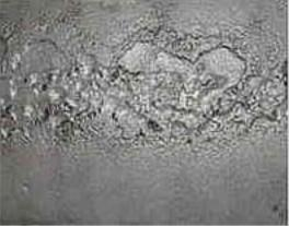
Fig 2: Image presenting the trend towards channel style corrosion. The channels were initially small pits that joined together and continued to grow. This type of corrosion pattern can result in defects with significant depth and length.
