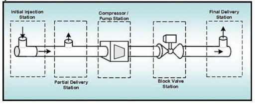
Fig. 4. Pipeline components
