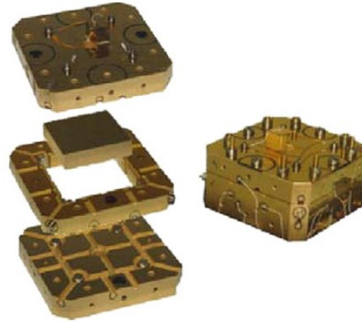
Fig. 1. GRACE accelerometer mechanical core
