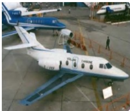
Fig. 4. The Falcon 10 S/N 005 with a wing made of carbon composite
