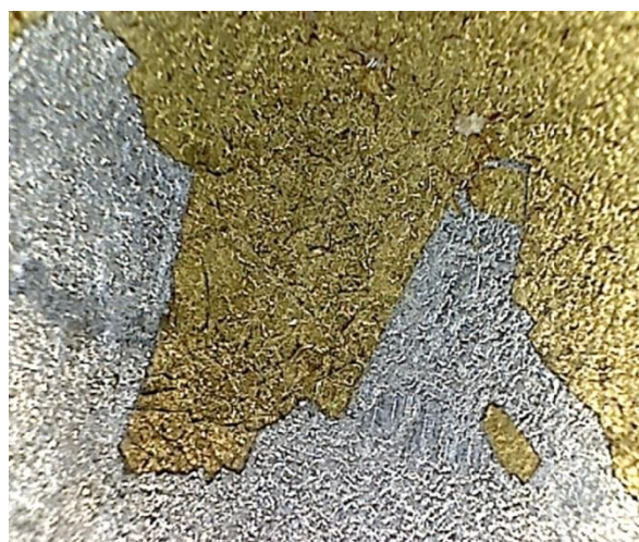
Fig.4 Coating, based on PR, obtained after 90 min, concentration under 150 °C
