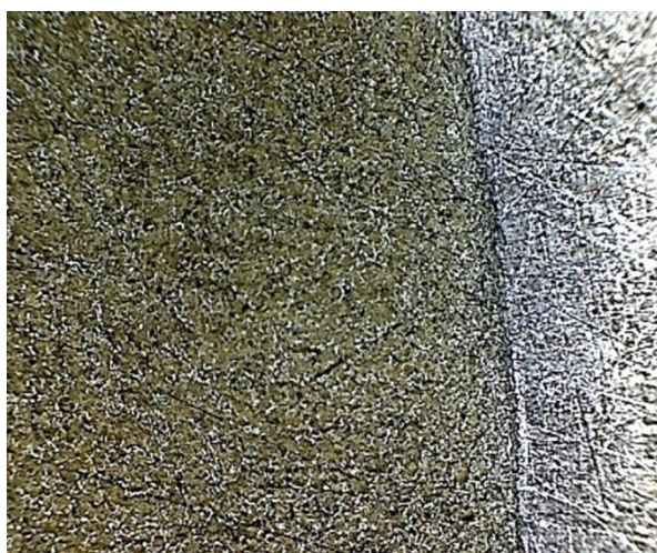
Fig.3 Coating, based on PR, obtained after 60 min, concentration under 150°C
