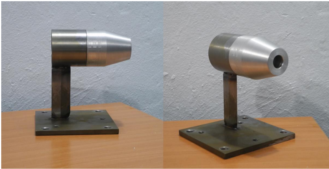
Fig. 2. Photos axisymmetric model of rocket-ramjet engine
