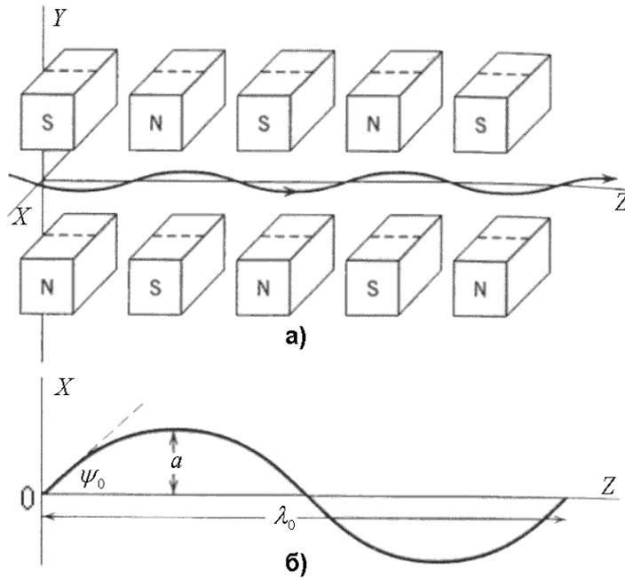
Fig. 31.1. The scheme of the flat undulator
