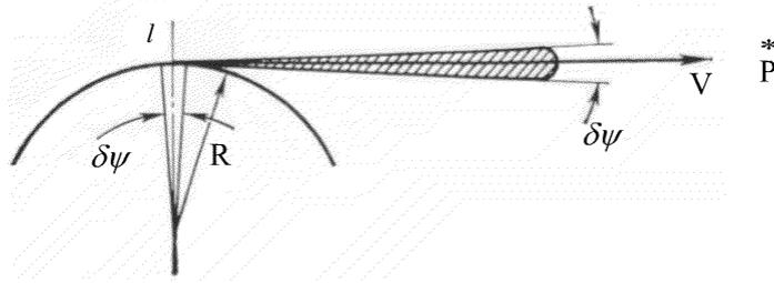
Fig. 25.3. The scheme of generation and registration of synchrotron radiation
