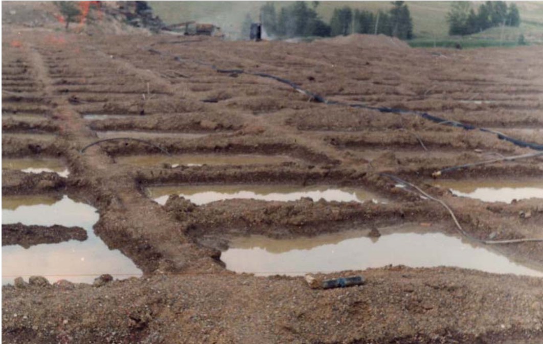
Fig. 46. Net of pond cells in the upper part of heap where cyanide solution is fed along the pipes. The solution leaks into crushed loose material and leaches Au. Ponds are filled as solution decreases. It is a so called pond method. There is also a spraying method (a specific shower for «heap»)
