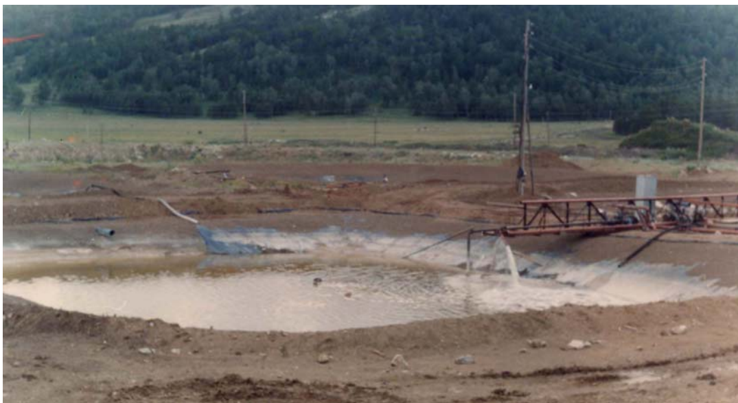
Fig. 47. Storage pond with cyanide solution from which gold has already recovered. Next, solution is reproduced to the necessary parameters and again is fed to heap (closed cycle). The plants of such kind uses only closed system of solution processing
