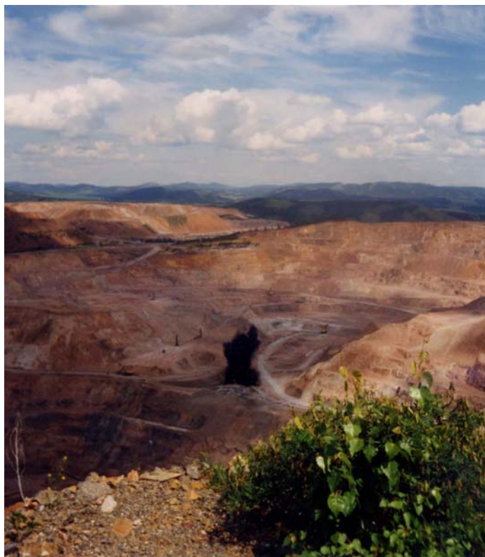
Fig. 40. The moment of explosion (dark column) at quarry of Sorsk Cu–Mo-field
