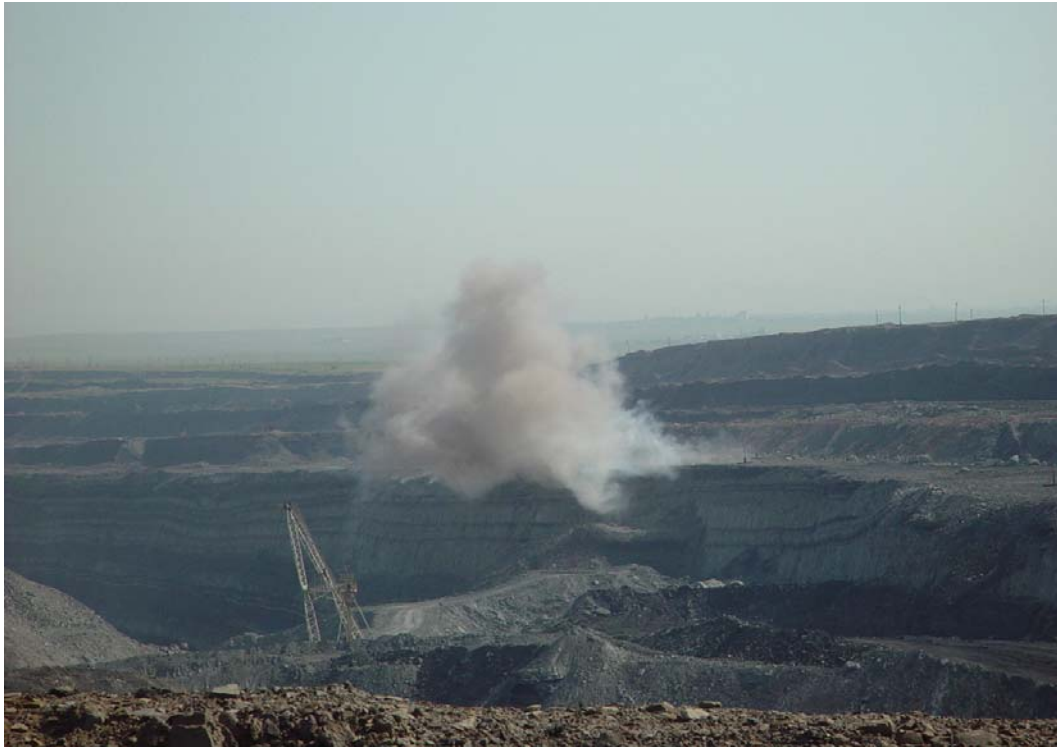
Fig. 52. Explosion at Vostochno-Beysk open-pit mine. One can see a dust and gas cloud
