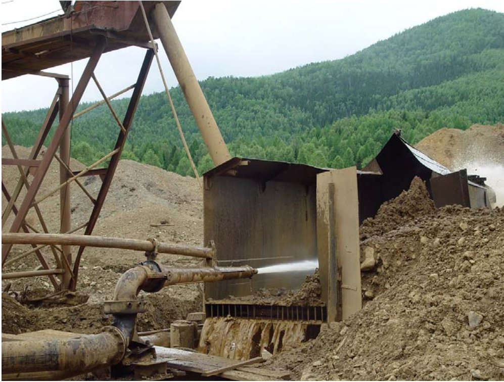
Fig. 27. Hydraulic giant operation at sand washing
