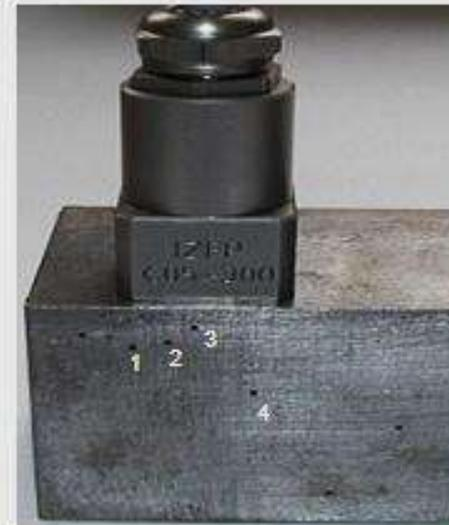
Partial View of Test Specimen with Transducer
