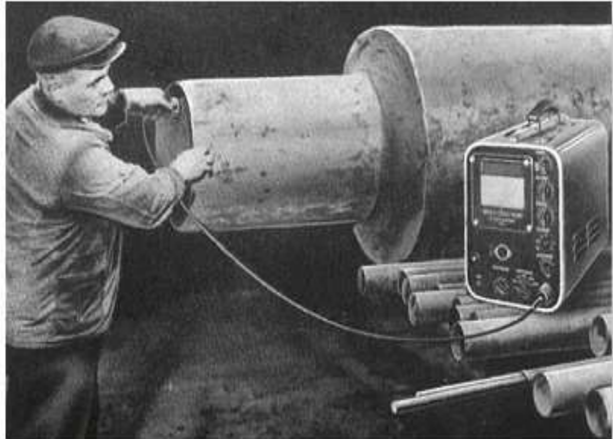
Early pipe testing with Krautkrämer apparatus (1950s)
