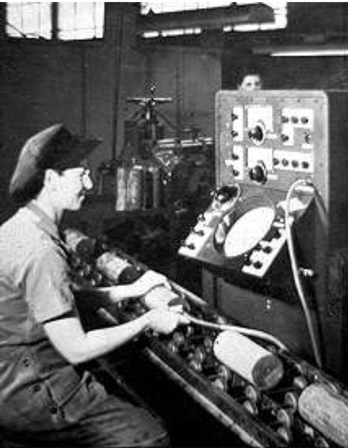
The 'Supersonic' UT unit, which was one of the first.
