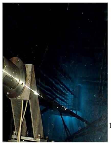
Flux of Thermal Neutrons in central channels: 1,7·10<sup>14</sup> n/(cm<sup>2</sup>·s) in peripheral channels: (2- 5)·10<sup>13</sup> n/(cm<sup>2</sup>·s)
