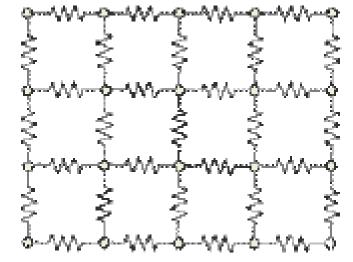
**Spring Model of Vibrating Particle Masses**
