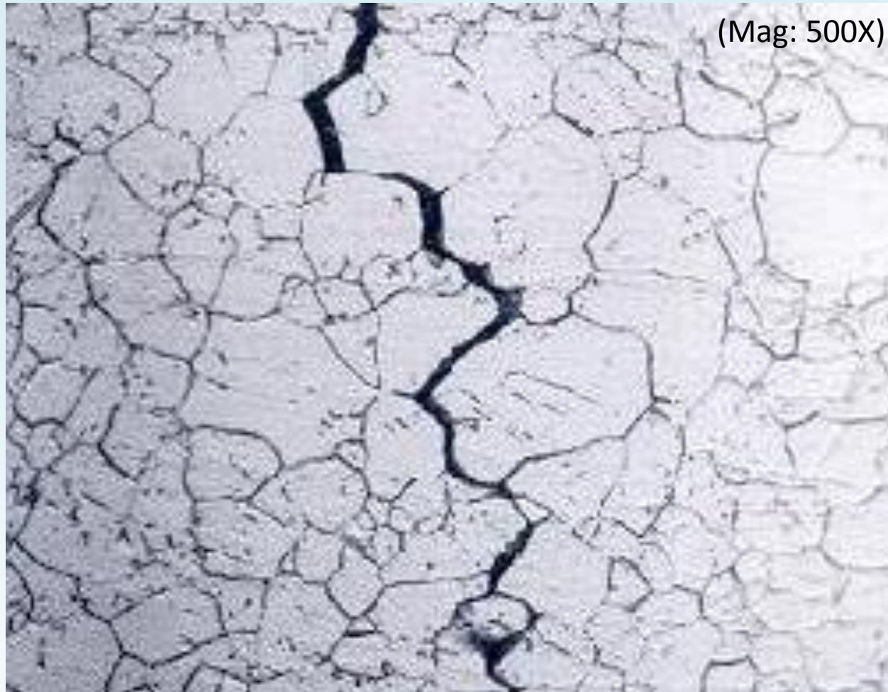
View of intergranular stress corrosion cracking (IGSCC) in an Inconel heat exchanger tube.
