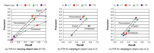
Fig. 5. Precision and recall for the three recommendation algorithms under different parameters settings.
