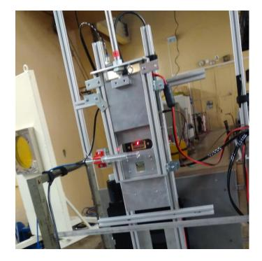
Positioning stage with connected ALPIDE chip
