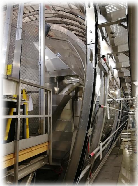
200-ton spectrometer for experiment KATRIN
