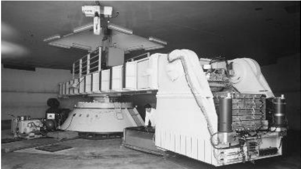
Figure 6.41. Geotechnical centrifuge at UC Davis. Note laminar box in centrifuge bucket for testing models under seismic loading conditions
