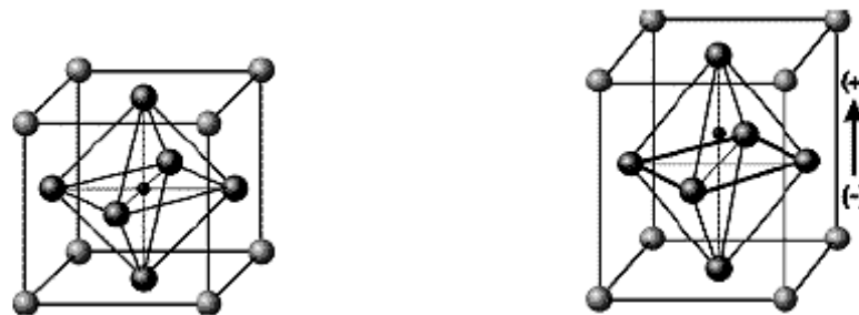
Figure 6.46 a) cubic lattice, symmetric arrangement of positive and negative charges. b) tetragonal (orthorhombic) lattice, crystal has electric dipole.
