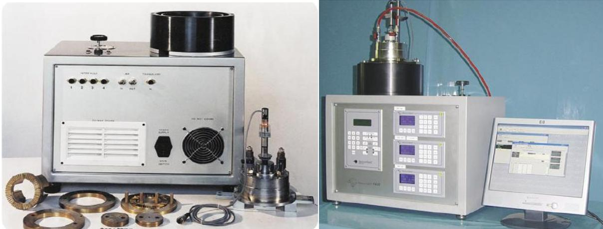
Figure 5.19. The Tecnotest's apparatus direct shear test on annular specimens
