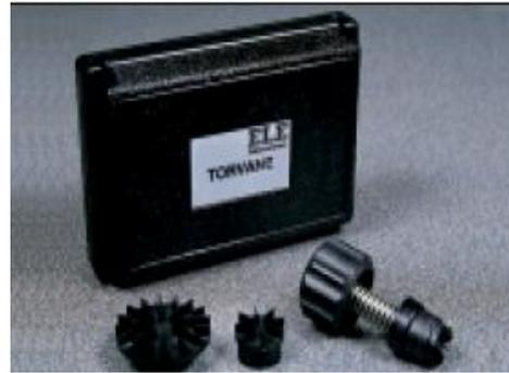
Figure 5.21. Pocket shearmeter
