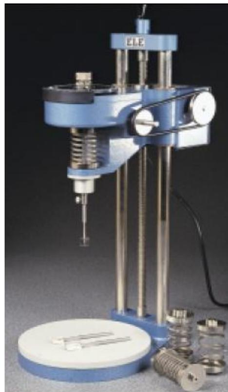
Figure 5.23. Laboratory vane apparatus and accessories
