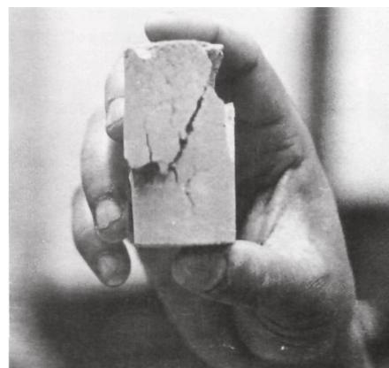
*Figure 5.30. A soil specimen after failure*
