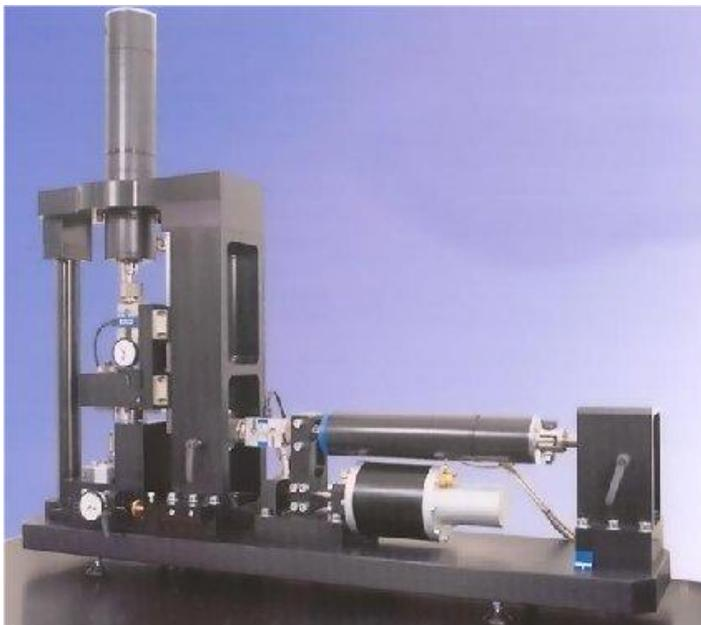
*Figure 5.18. The direct simple shear apparatus*
