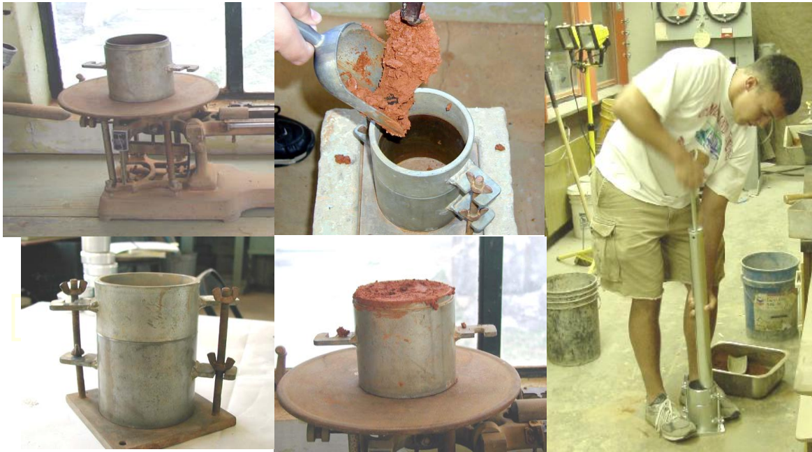
Figure 2.4. Procedure of soil preparation for compaction tests
