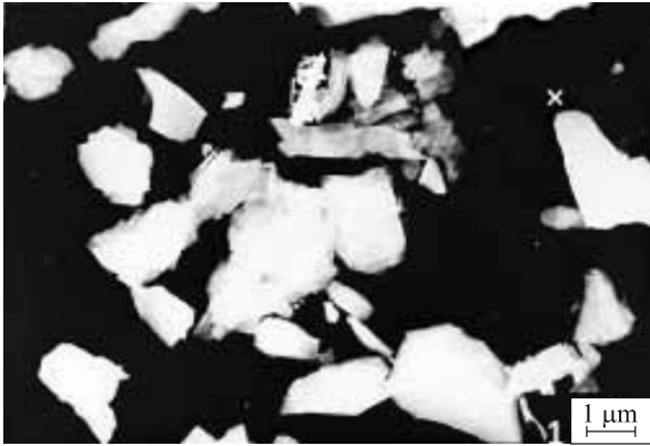
Fig. 1. Electron micrograph of pyrophyllite rock. \times 5000 .
