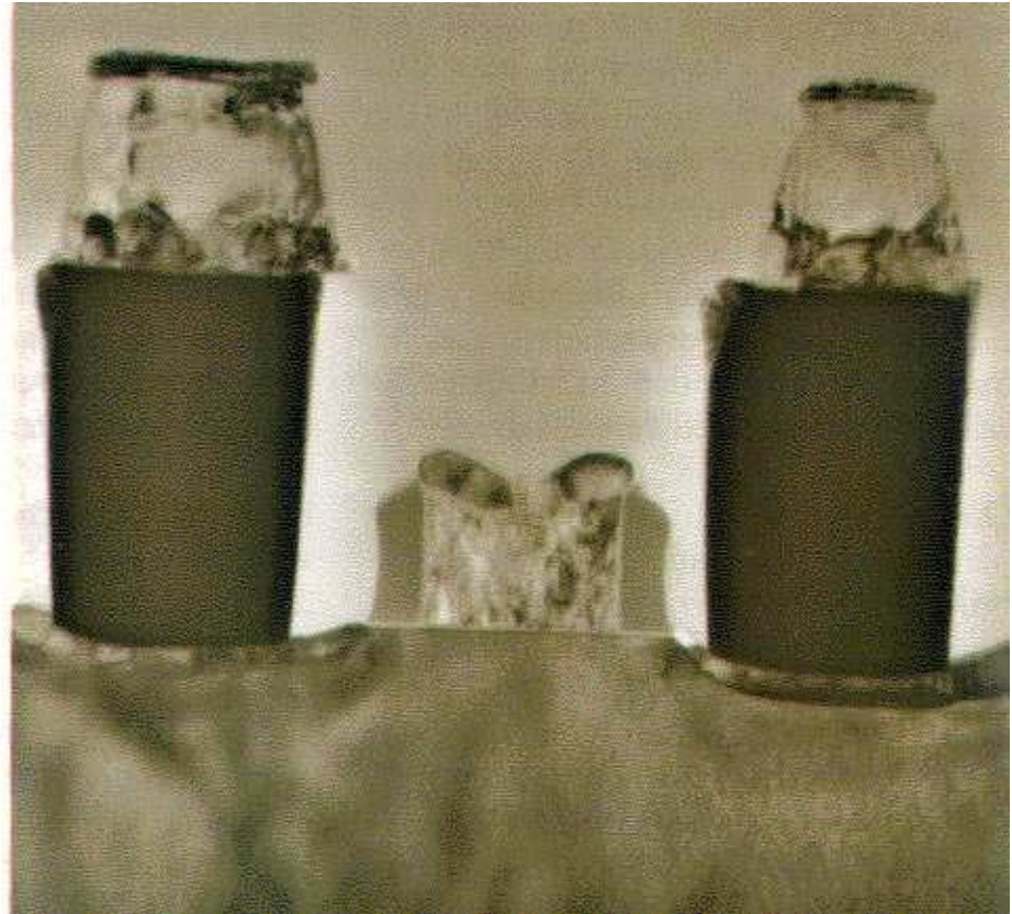
1995: transistor structures between 0,4 and 1,3 \mu\text{m}
