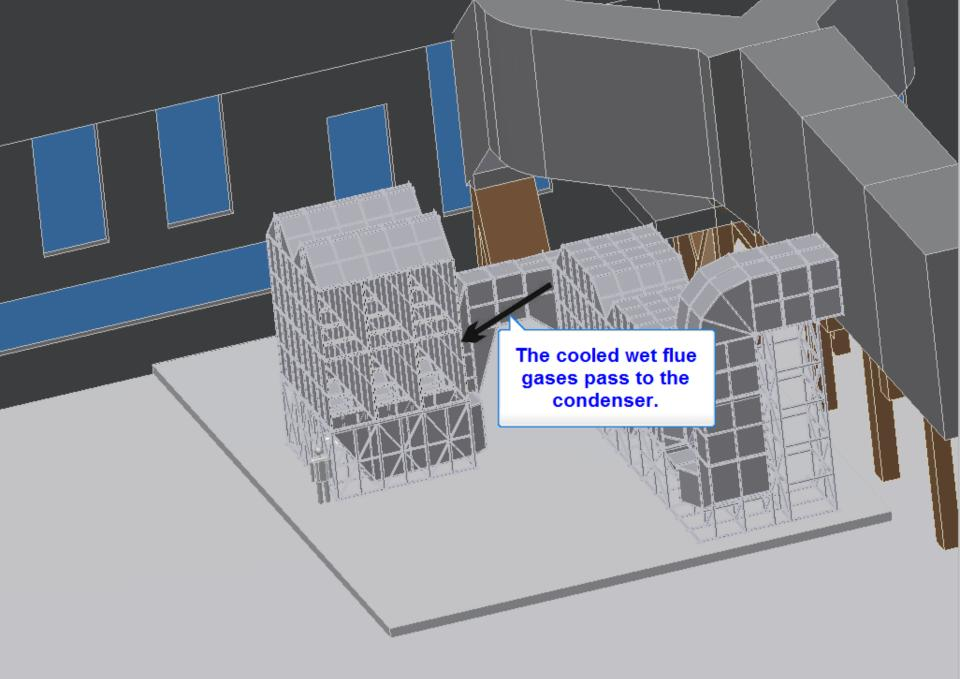
The water vapor condenses when the wet flue gases pass through the condenser's tunnels.
