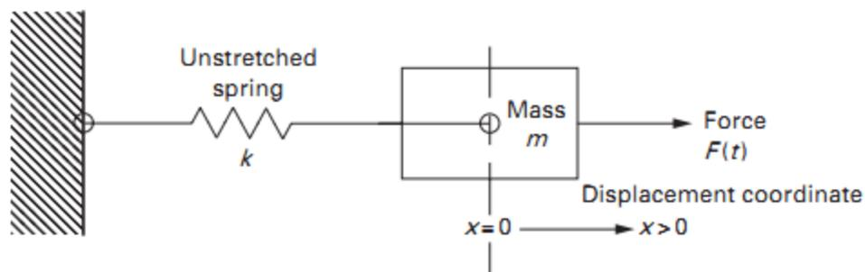
Figure 6.1 An elementary *spring-mass system* the shows an ideal spring exerting a restoring force on a mass,  $m$ , as does a specified applied force,  $F(t)$ . The spring's stiffness is  $k$ , and the displacement or movement of the mass to which the spring's right end is attached is  $x(t)$ .
