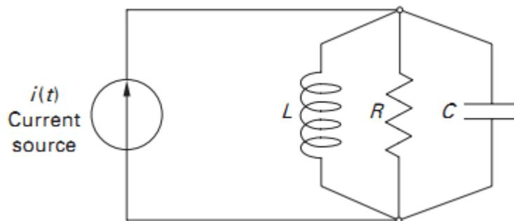
Figure 6.3 A *parallel RLC circuit* that has a current source as its driver. The elements are the *capacitor* of capacitance,  $C$ , the *inductor* with inductance,  $L$ , and the *resistor* with resistance,  $R$ . The current source provides a current of magnitude,  $i_{\text{source}}(t)$ .
