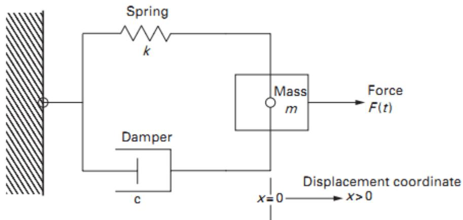
Figure 6.2 An elementary *spring-mass-damper* system that shows the ideal spring (of stiffness,  $k$ ) exerting a force on a mass,  $m$ , the specified applied force,  $F(t)$ , and a viscous damping element that exerts a restoring force that is proportional to the speed,  $\dot{x}(t)$ , at which the mass moves.
