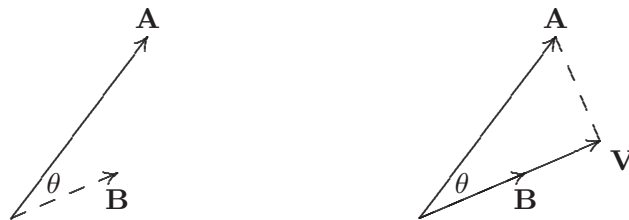
Figure 11.7 \mathbf{V} is the projection of \mathbf{A} onto \mathbf{B} .
