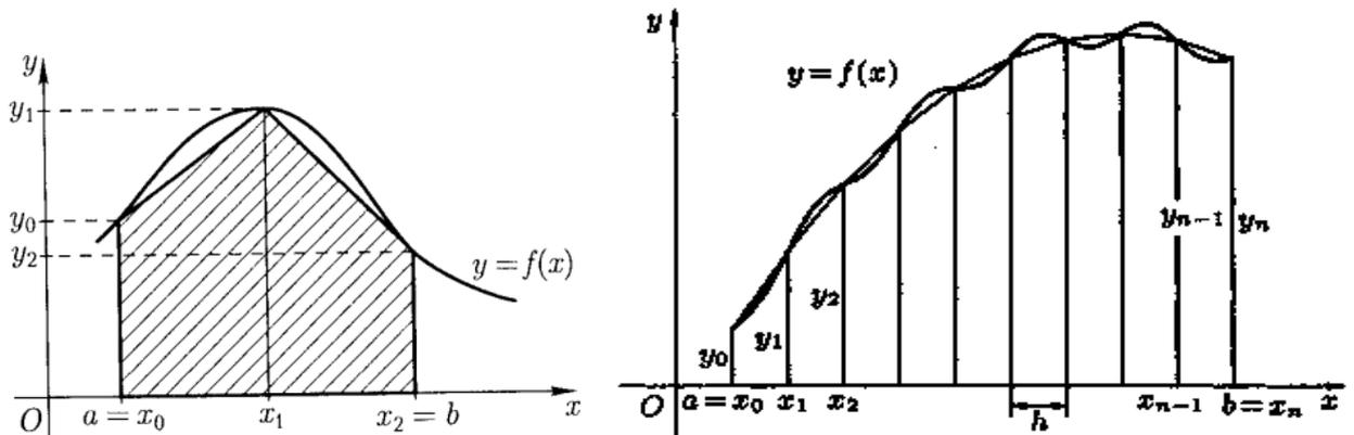
$$\int_a^b f(x) dx \approx h \frac{y_0 + y_1}{2} + h \frac{y_1 + y_2}{2} + \dots + h \frac{y_{n-1} + y_n}{2} =$$
