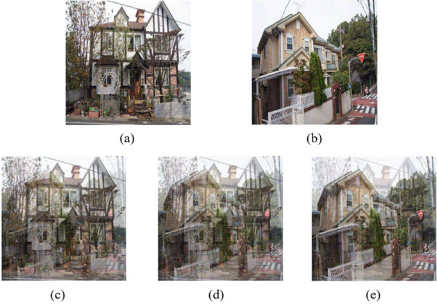
Fig. 2.8 Example of \alpha blending operation: (a) Image A; (b) Image B; (c) T_\alpha = 178 ; (d) T_\alpha = 128 ; and (e) T_\alpha = 77
