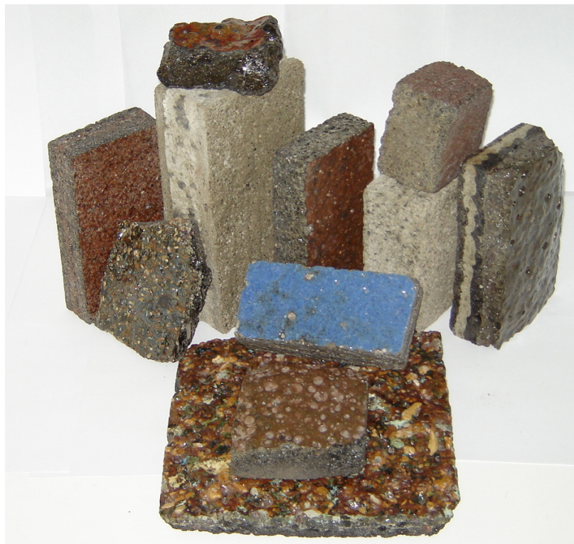
Picture 1. Constructional heat-insulating material "Viralit" of different types
