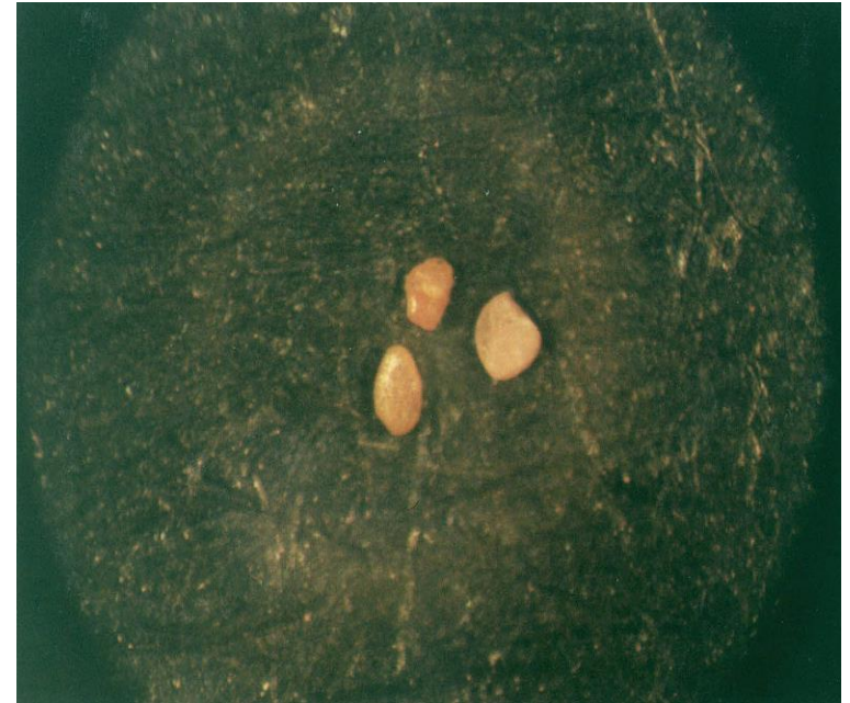
Feldspar – small, right- angled, pink (feldspar) Size ranges from 28 \mu\text{m} to 500 \mu\text{m} .
