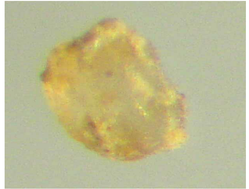
Quartz covered by iron oxides – translucent, partly gravel. Size ranges from 28 \mu\text{m} to 1 mm.
