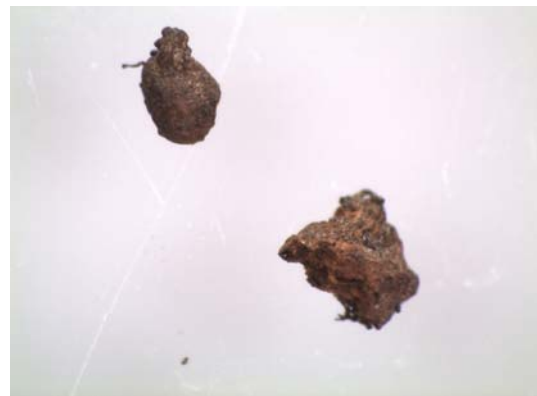
Fig. 3.3.5.5. Iron oxides (binocular, magnification 50 x ) (Жорняк, 2009)
