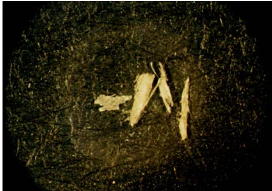
Fig. 3.2.4.20. Woodwork particles (from 140\mu\text{m} to 1\text{mm} ) (binocular, magnification 50\times )
