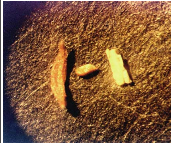
Fig. 3.2.4.4. Vegetable particles (0,1...0,6 mm) (binocular, magnification 50 x )
