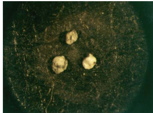
Fig. 3.2.4.25. Grey semirounded particles (14...520 \mu\text{m} ) (binocular, magnification 50 x )
