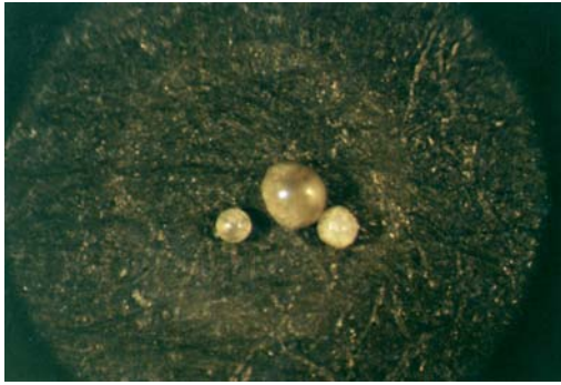
Fig. 3.2.4.10. Microspherules of silica-alumina composition (binocular, magnification 50 x )
