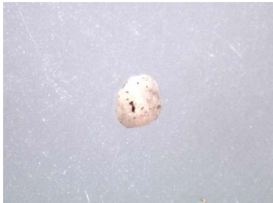
Fig. 3.3.5.4. Carbonate particle (binocular, magnification 50 x ) (Жорняк, 2009)
