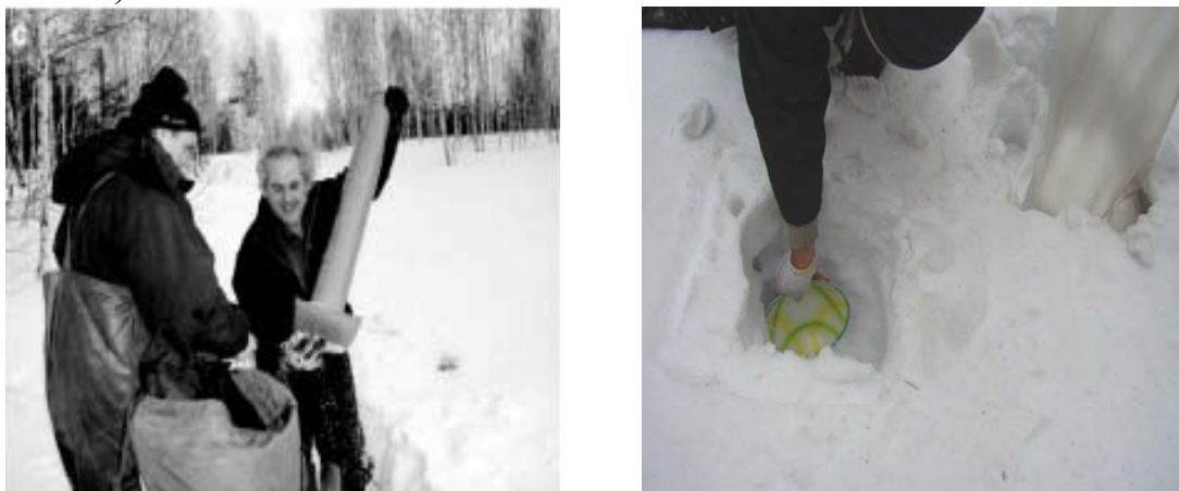
Fig. 3.2.2.1 Snow sampling (left – by snow sorter (V. Udachin), right – pit method)
