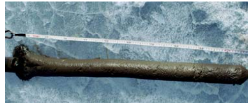
Column of bottom sediment
