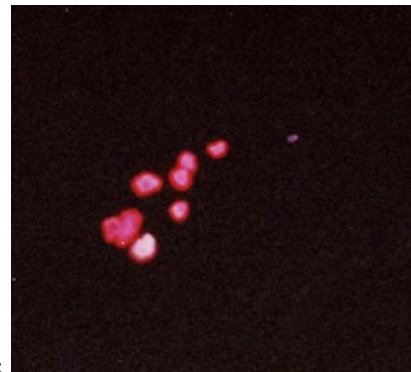
Fig. 3.2.4.5. Particles of feldspar (from 28 \mu\text{m} to 1mm): a) under a binocular microscope (magnification 50 x ); b) under an electron microscope (magnification 8 K x ); c) energo-dispersive spectrum; d) results of impulsive cathodic luminescence
