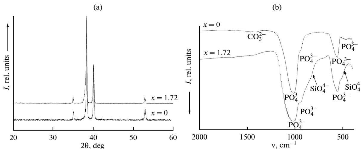
Fig. 4. (a) X-ray patterns and (b) IR absorption spectra of coatings grown by RF magnetron sputtering.
