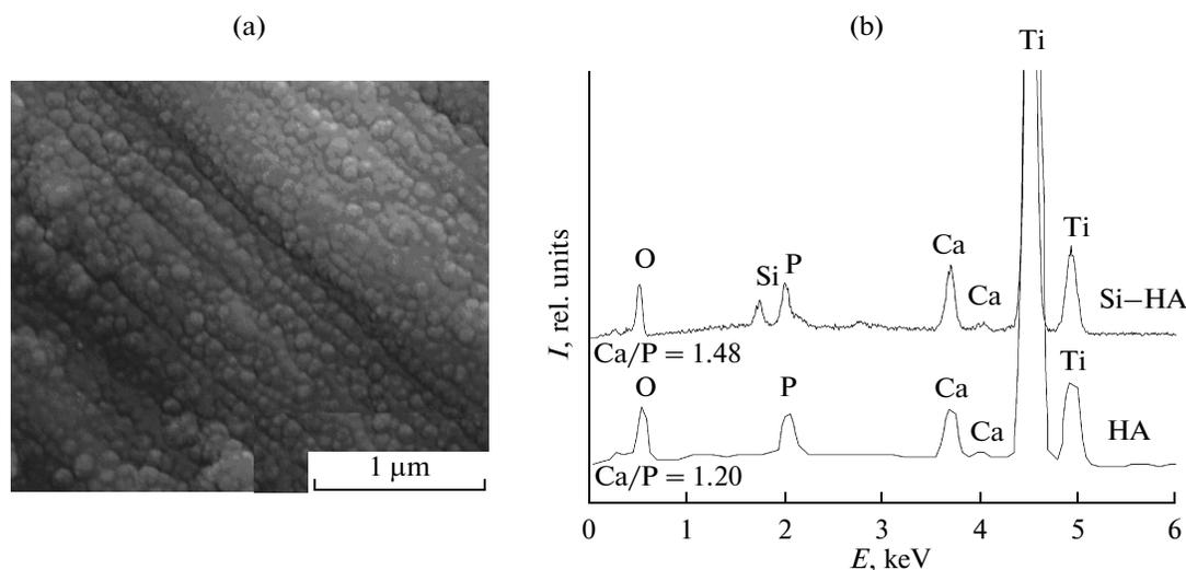
Fig. 2. (a) SEM image of the surface and (b) EDX spectra of coatings grown by RF magnetron sputtering.
