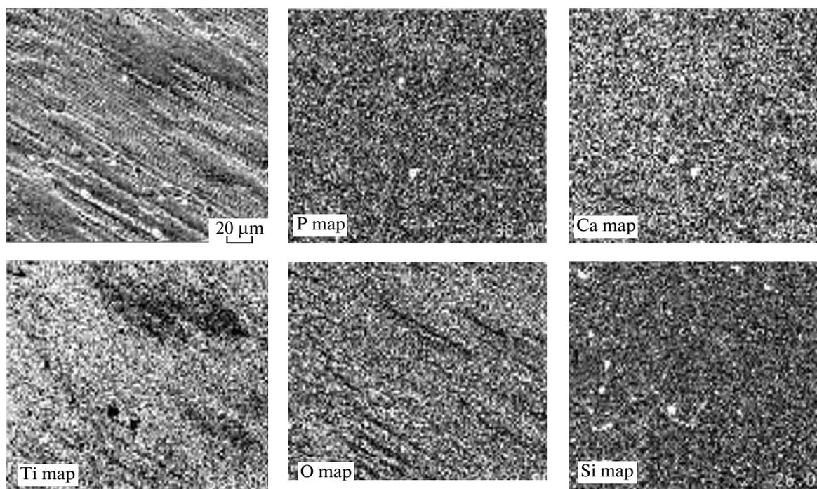
Fig. 3. Maps of element distributions in Si-CaP coatings grown by RF magnetron sputtering.
