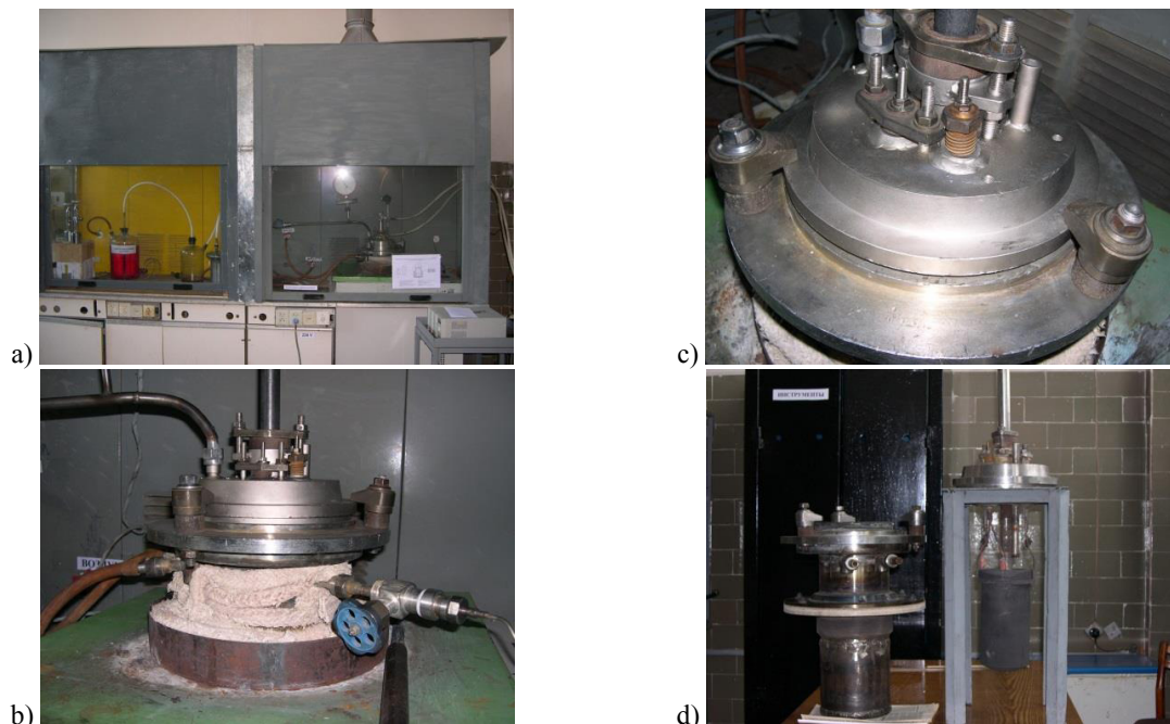
Fig. 2. Electrolytic installation for the electrolytic decomposition of titanium tetrafluoride: a) General view of the installation; b) tight electrolyser; c) the nickel-plated cover of the electrolyser; d) graphite crucible: the anode with current conductor (below), the metal cathode (above) and an electrolyser retort (at the left)
