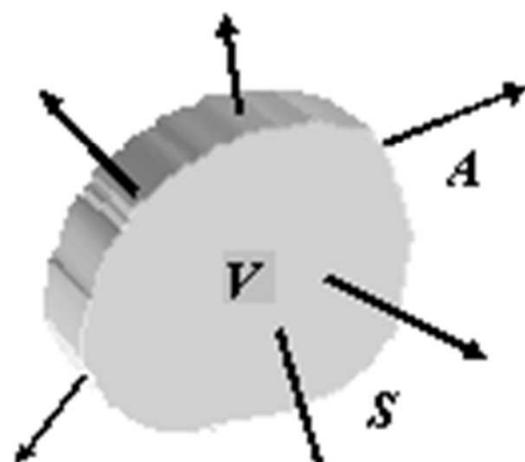
$$\lim_{\Delta V \rightarrow 0} \frac{\Delta N}{\Delta V} = \frac{dN}{dV} = \text{div} \vec{A}$$
