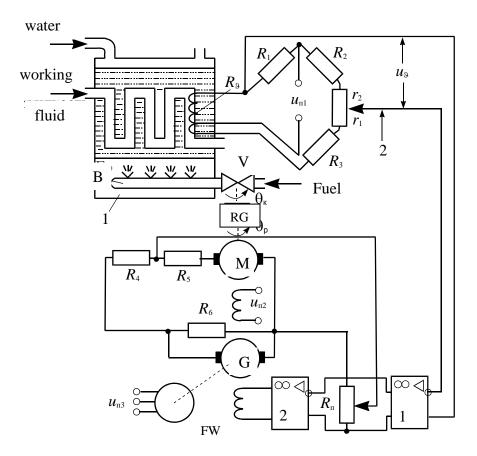
Thermometer  $R_{\mathcal{G}}$  changes its resistance according to the temperature of the working fluid flowing in the pipeline through the furnace 1. Move the slider of the set point 2 and break bridge balance.
