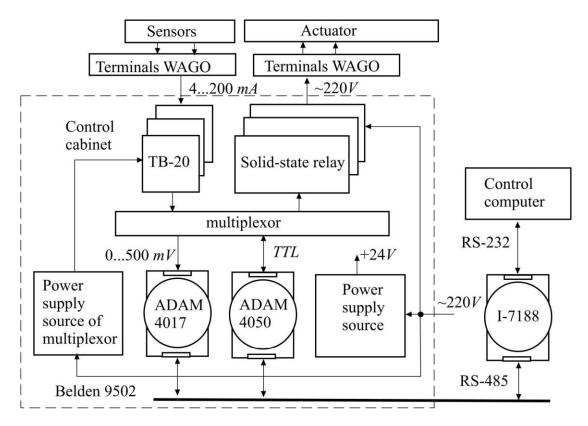
Control functions are performed by a channel controller I-7188 which has 256 KB of RAM, flash memory is 512 KB, console port, serial ports RS-232 and RS-485, a watchdog timer, real time clock and it is compatible with an operating system ROM-DOS. A controller is connected to a control computer through RS-232, and via an RS-485 cable (Belden 9502) it is connected to a control cabinet.
