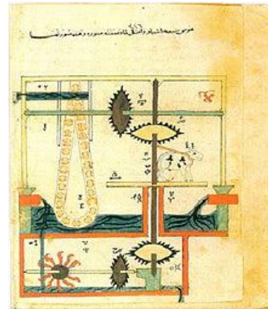
Fig. 1.1. Al-Jazari's hydropowered chain pump device
