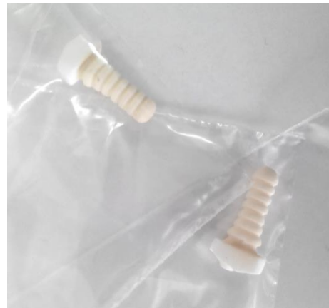
Ceramic samples with CaP coating
