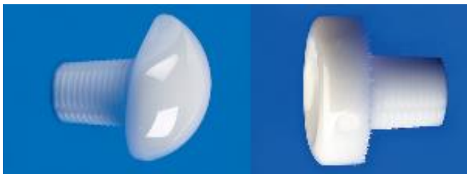
Ceramic samples without CaP coating
