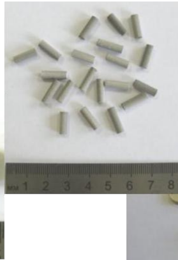
Ceramic samples with CaP coating
