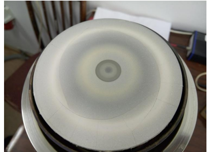
Erosion on the target surface
