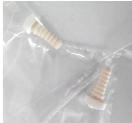
Ceramic samples with CaP coating
