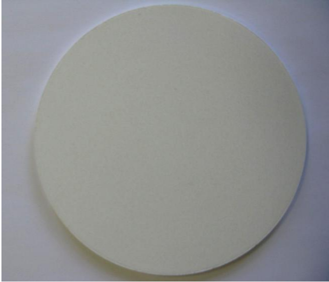
Target for sputtering made from pure hydroxyapatite powder
