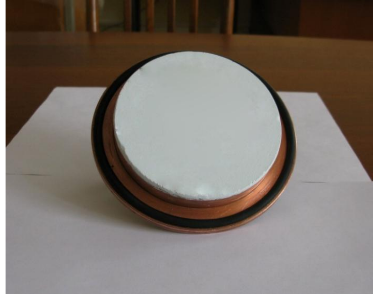
Magnetron with cathode from hydroxyapatite
