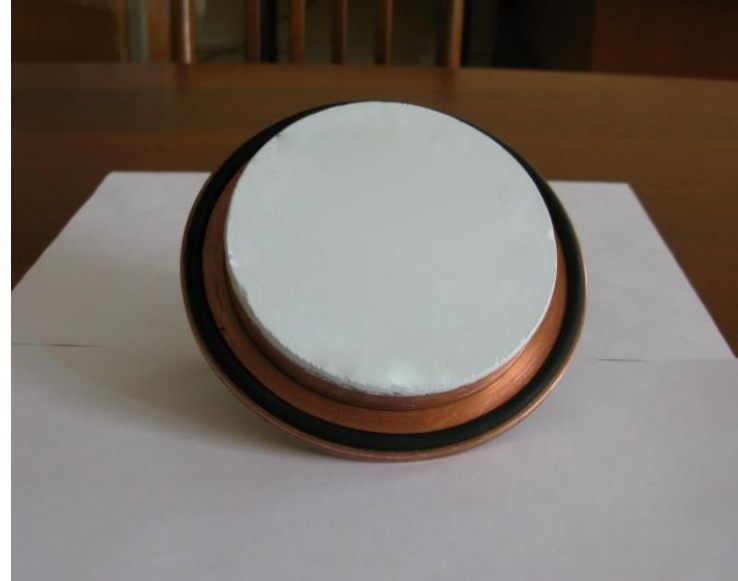
Magnetron with cathode from hydroxyapatite
