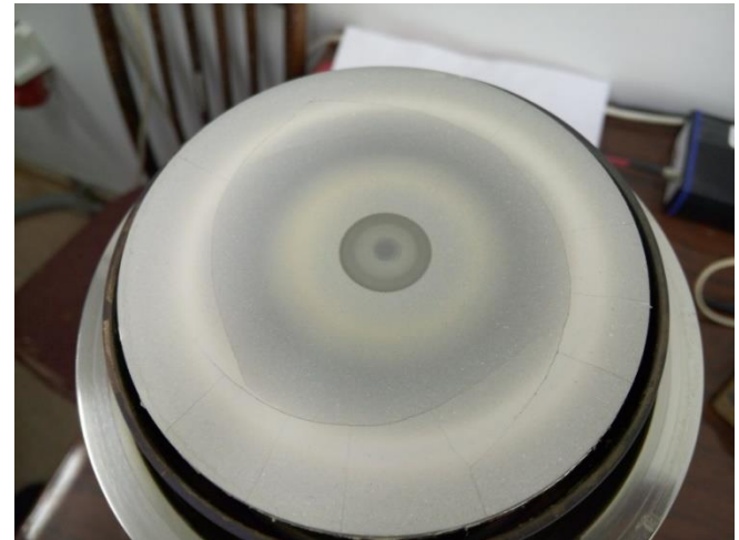
Erosion on the target surface
