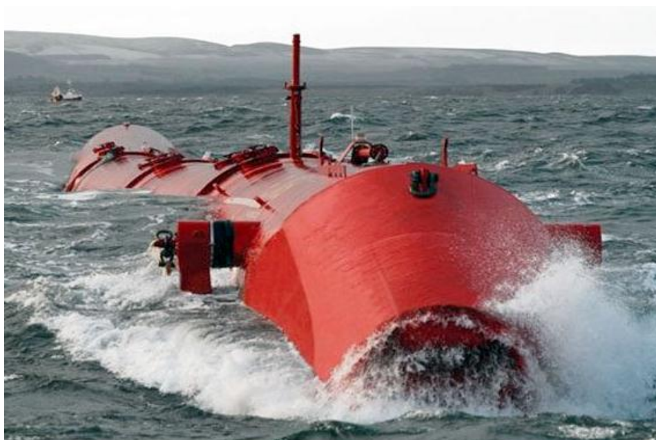
Рис. 7.4. Коммерческая волновая электростанция ( https://www.thescottishsun.co.uk/news/scottish-news/2097759/scot-gov-prize-worth-10million-for-wave-energy-machine-sinks-without-trace/amp )
