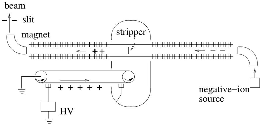
**Fig. B.2.** A schematic of a tandem Van de Graff accelerator. Negative ions are accelerated to the positive potential where a “stripper” removes electrons. The resulting positive ions are then accelerating to ground potential where a definite charge state is selected by a magnetic field and slit.
