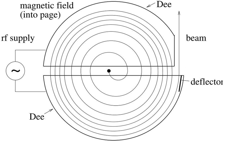
**Fig. B.5.** Schematic of a cyclotron. Particles are injected near the center of a dipole magnetic field and then spiral outward as they gain energy each time they pass through the alternating electric field between two electrodes called “Dee’s.” The radio-frequency is tuned to the particle’s cyclotron frequency,  $\omega_c = qB/m$ . Near the maximum radius, the particles are deflected out of the cyclotron.
