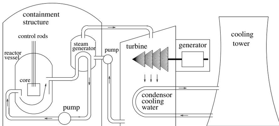
Fig. 6.10. Schematic of a pressurized water reactor.
