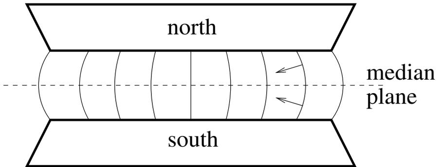
**Fig. B.6.** Vertical focusing in a radially-decreasing dipole magnetic field. Particles in the median plane experience a horizontal force. The force on particles above or below the median plane has a vertical component that pushes the particle back toward the median.
