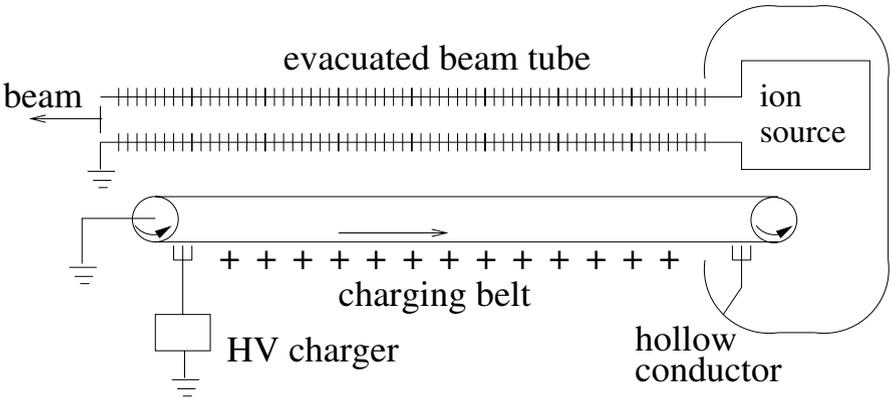
**Fig. B.1.** A schematic of a simple Van de Graaff accelerator. Positive charges are transferred from ground potential to a hollow terminal. The ion source is placed inside the terminal and particles are accelerated through the electrostatic field to ground potential.
