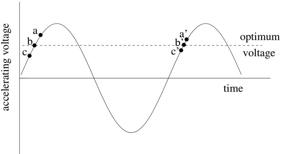
**Fig. B.4.** The principle of phase stability in a linear accelerator. Particles arriving in a gap at point b are accelerated such that they arrive at the text gap at the point b' with the same phase with respect to the alternating field. Particles arriving at point a (c) receive more (less) acceleration and therefore arrive relatively earlier (later) in the next gap, point a' (c'). Particles in the range a-c are thus “focused” in phase-space toward the point b.
