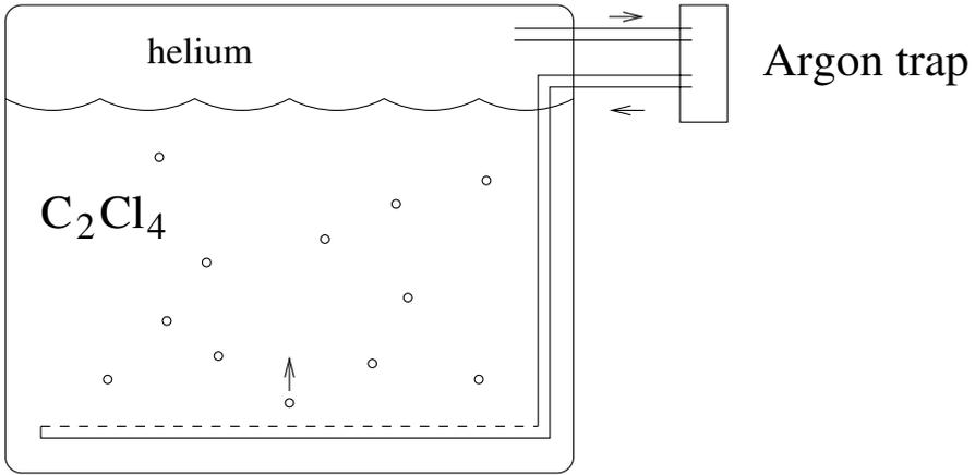
**Fig. 8.17.** The principle of the Homestake neutrino experiment.  $^{37}\text{Ar}$  atoms produced by neutrino absorption are swept out of the  $\text{C}_2\text{Cl}_4$  by bubbling helium gas through the liquid. The argon is then separated in a cold trap and introduced into a small proportional counter where the electron-capture decays of  $^{37}\text{Ar}$  are observed
