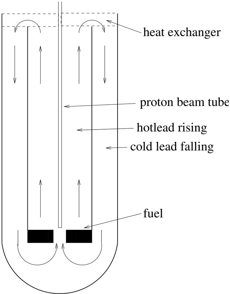
**Fig. 6.14.** A possible design of a hybrid reactor [66]. The proton beam is directed downward entering a region containing molten lead and surrounded by thorium fuel. The neutrons created in the lead induce fission in the thorium. The heat generated causes the lead to rise toward heat exchangers.
