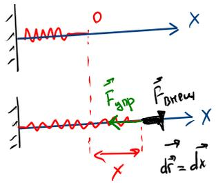
$$|\vec{F}_{\text{уп}}| = k \cdot x \quad \vec{F}_{\text{уп}} \uparrow \downarrow d\vec{r} \Rightarrow \alpha = 180^\circ$$
