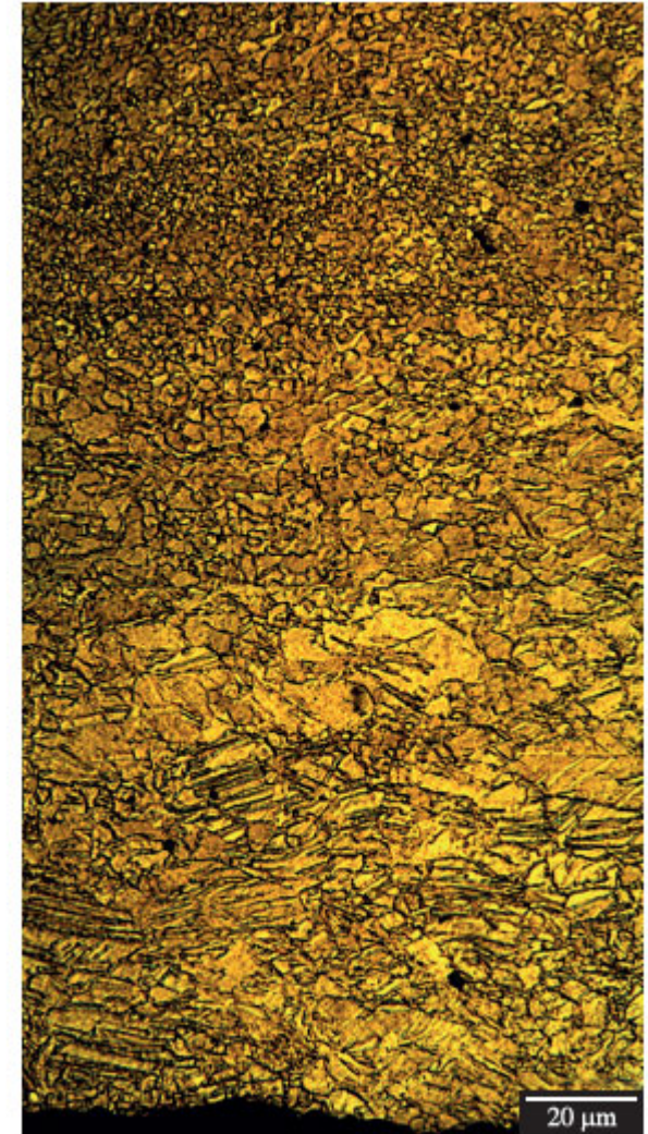
Figure 2. Grain structure in the region near the bottom of a sample processed by HPT for 1/4 turn at 463 K 12 .
