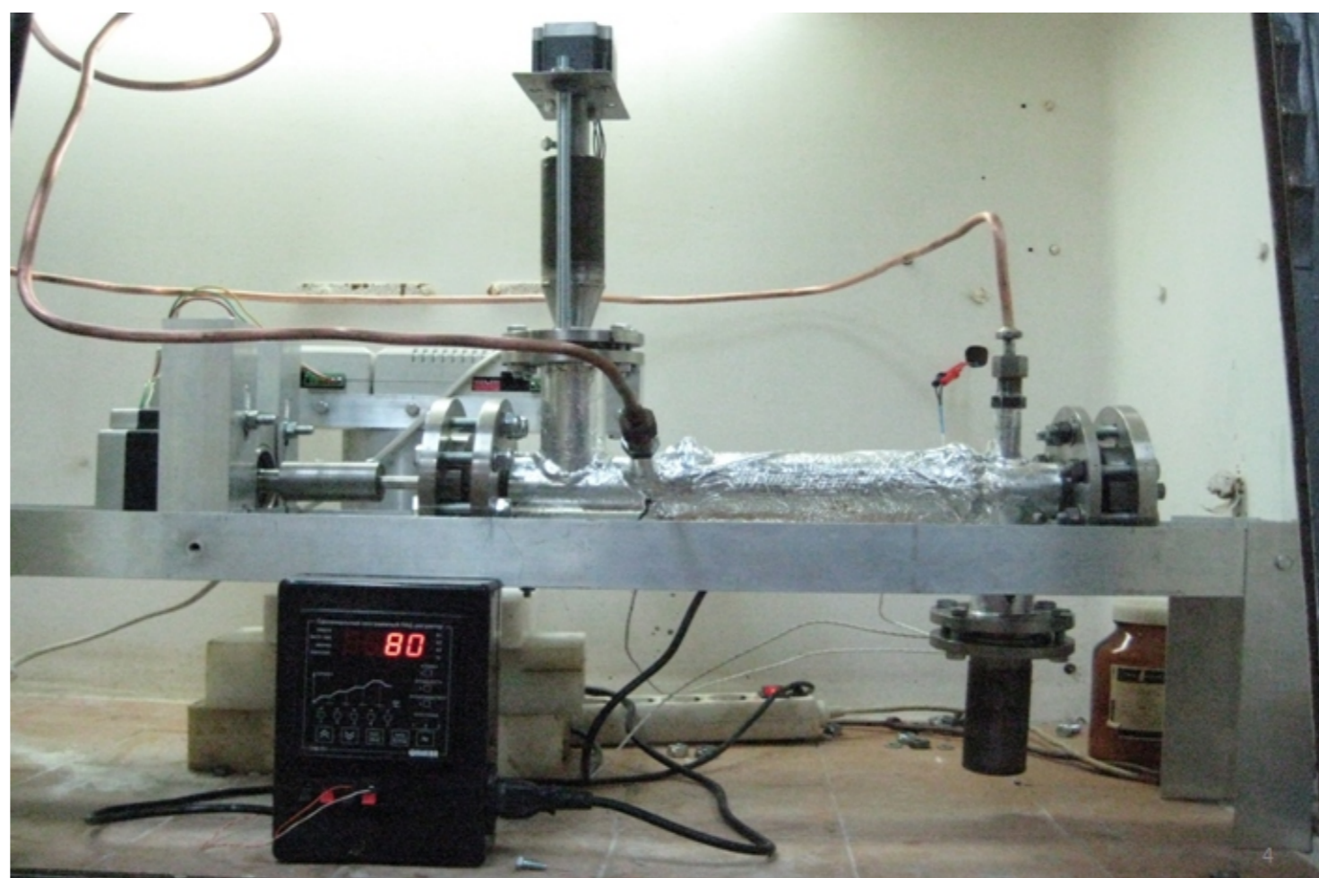
Assemble drawing, of the horizontal reactor for the fluorination of potassium bromide
