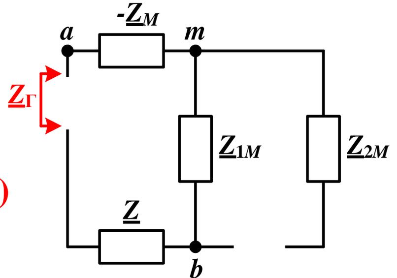
$$\underline{Z}_\Gamma = -\underline{Z}_M + \underline{Z}_{1M} + \underline{Z} = 50 = 50e^{j0^\circ} \text{ (ОМ)}$$
