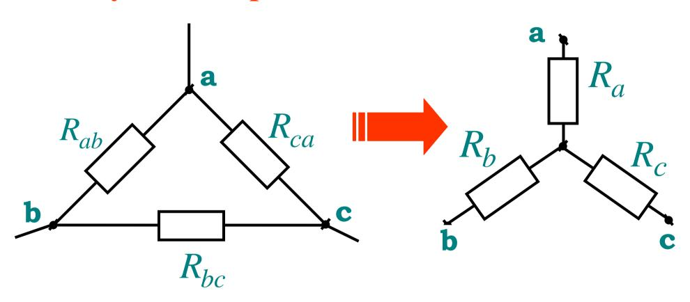
$$R_a = \frac{R_{ab}R_{ca}}{R_{ab} + R_{bc} + R_{ca}}$$
