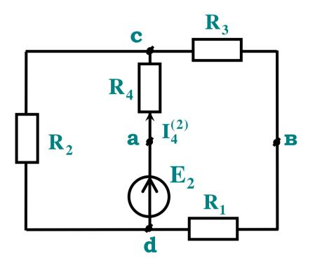
$$I_4^{(2)} = \frac{E_2}{R_4 + \frac{R_2(R_1 + R_3)}{R_2 + (R_1 + R_3)}}$$
