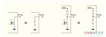
Режим **open-drain**. Справа open-drain, with pull-up
