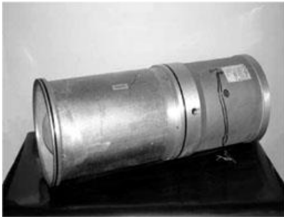
Fig . 3.75. Measurement transducer of gas turbine TRZ meter
