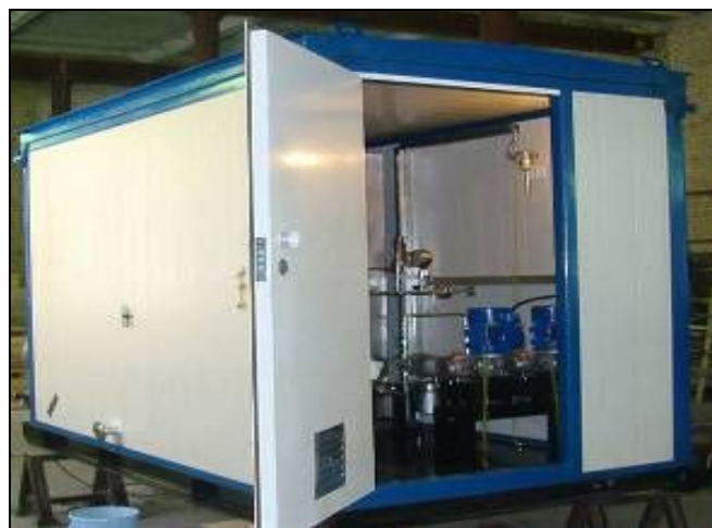
Fig. 16. General view of dosage chemical agent unit “Ozna Batcher” in a heated room
