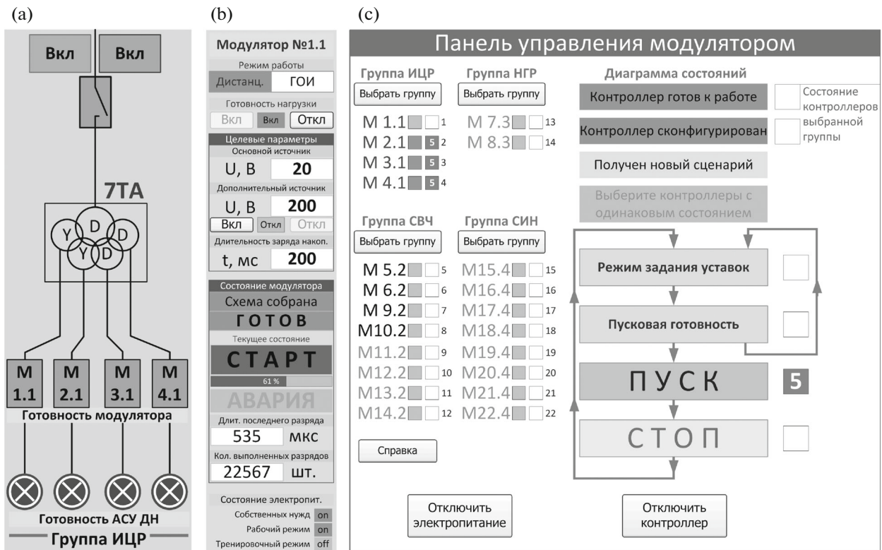
Fig. 5. Appearances of the graphical forms: (a) control and monitoring of the power supply of the modulators; (b) monitoring and input of modulator parameters into the MCU; (c) input of control commands of the MCU in accordance with the state diagram with consideration for admissible jumps. The designations on the panel of the auxiliary heating system: (IC) ion-cyclotron heating, (MCW) microwave heating, (LHR) low-hybrid resonance heating, and (INJ) injection heating.
