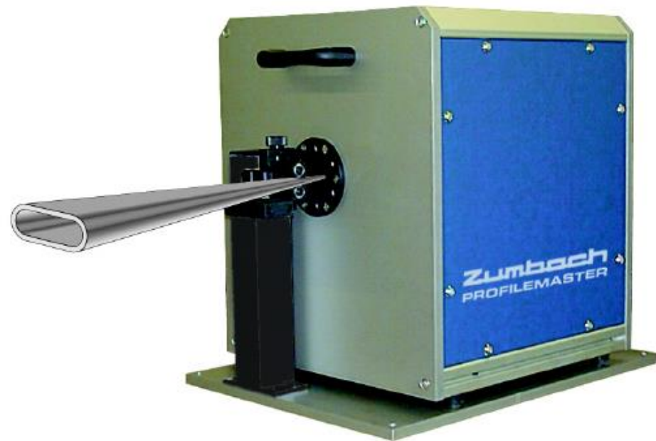
Pictures shows: PROFILEMASTER Measuring Unit
